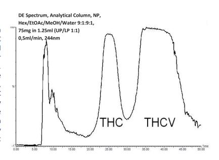
Following chromatography, fractions collected between 32 and 46 minutes were combined and concentrated, in vacuo, to yield >90% recovery of >98% pure, THCV. Further method development culminated in a 1g scaled loading and the use of scaled run conditions on the Spectrum preparative column in Reverse Phase Mode. This experiment produced >90% recovery of >97% pure THCV. This separation was effectively completed in less than thirty minutes.
