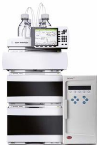
Figure 1. HPLC Agilent 1260 Infinity series coupled with a Decade Elite Electrochemical Detector used in this study.
