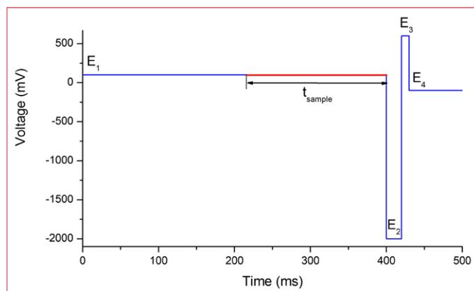
**Figure 1:** 4-step PAD potential waveform for the detection of Ethylene glycol.
