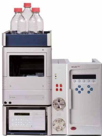
Figure 1: ALEXYS analyzer for FDG with AS 110 autosampler.
