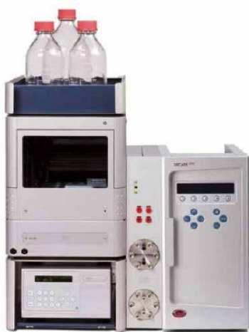
Figure 1: ALEXYS analyzer for FDG with AS 110 autosampler.
