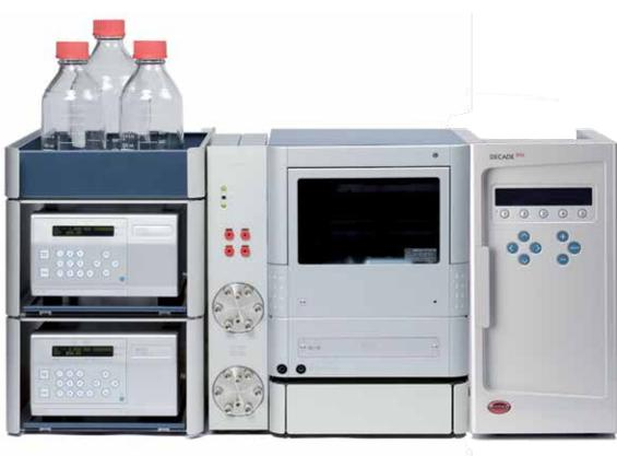
Figure 1: ALEXYS HPAEC-PAD analyzer with binary gradient for  $\beta$ -cyclodextrins.
