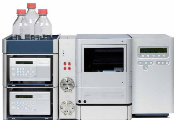
Figure 1: ALEXYS Aminoglycosides Analyzer for Spectinomycin.
