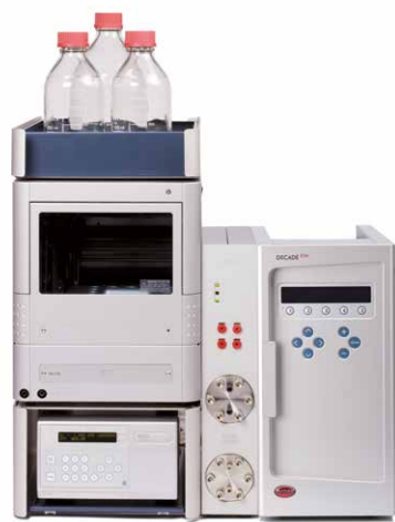
Figure 1: ALEXYS Macrolide Antibiotics Analyzer.
