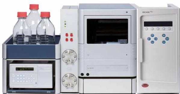
Figure 1: ALEXYS UHPLC/ECD Analyzer for Aminothiols and Disulfides.
