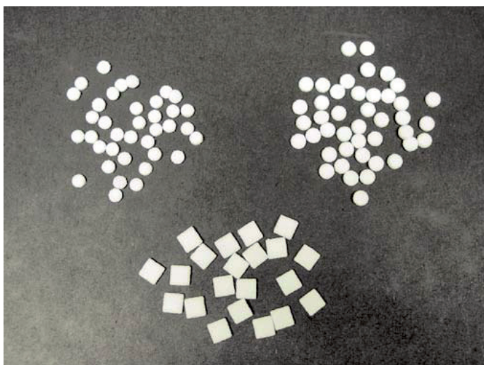
Frits to accommodate the 96 well plates.
